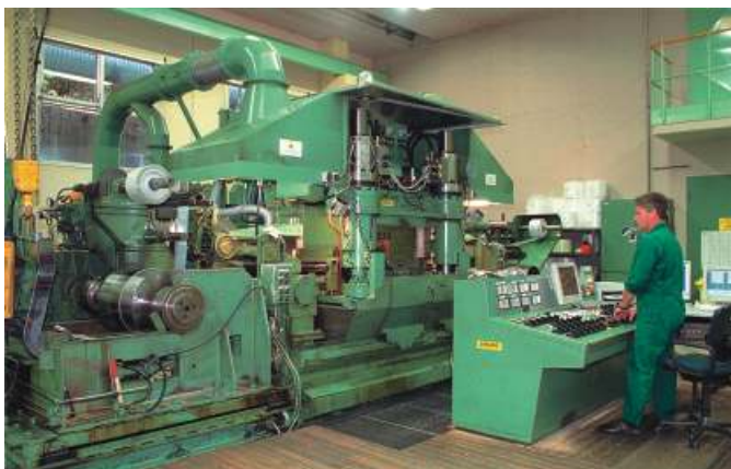
Control panel of the mill stand
